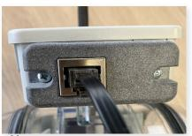
3/ Check the cable is well connected then do the same with the other e-VAV
