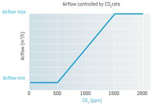
CO<sub>2</sub> min: 500 ppm  $\rightarrow$  airflow min CO<sub>2</sub> max 1500 ppm  $\rightarrow$  airflow max
