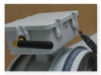
1/ Open the box with a flat screwdriver by unhooking the 4 clips
