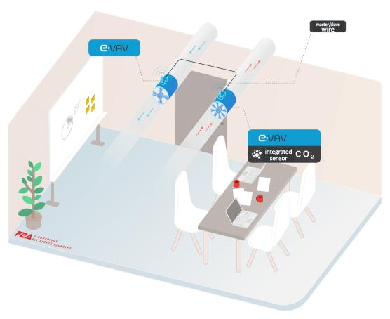
The **e-VAV QAI** damper in the exhaust is controlled by the  $CO_2$  measured from its integrated sensor. It is factory set with minimum and maximum airflow and  $CO_2$  values.
