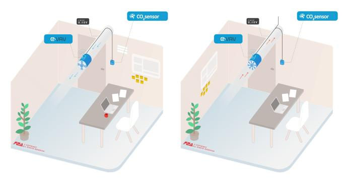
The damper is controlled by a  $0..10\,\mathrm{V}$  signal from a room  $\mathrm{CO}_2$  sensor which itself measures in real time the  $\mathrm{CO}_2$  concentration and sends a  $0..10\,\mathrm{V}$  signal to the damper to adapt the airflow rate.
