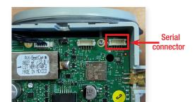
2/ Connect the connector to the « serial » port of the electronic board
