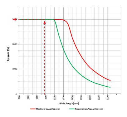
We recommend that the differential pressure does not exceed 3000Pa for a 1000-mm long M damper in galvanized steel.
