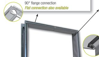
The ELYT+ is custom-made, from 240 x 240 mm to 2200 x 2200 mm with standard frame profiles of 20 or 30 mm. Bigger dimensions are provided with reinforced profiles and additional angle fasteners.
