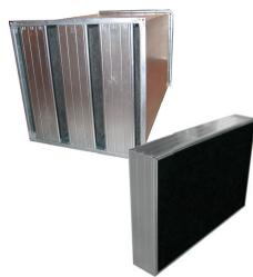
SONIE BS+ acoustic splitters are designed to be installed in aeraulic networks and enable to attenuate the noise generated by the ventilation system. SONIE BS+ splitters offer a better sound treatment for low frequencies: +10% attenuation between 250 & 500 Hz compared to standard splitters
