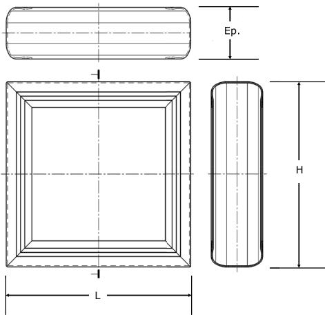
For larger dimensions, acoustic splitters are provided in several units with mounting accessories.
